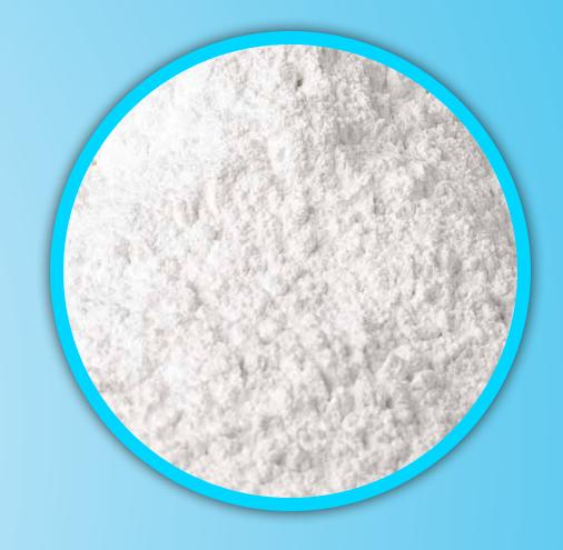
Hydrated lime is a dry fine, white powder with chemical formula Ca(OH)<sub>2</sub>.it is a type of dry powder made from limestone. It is created by adding water to quicklime in order to turn oxides into Hydroxides.
